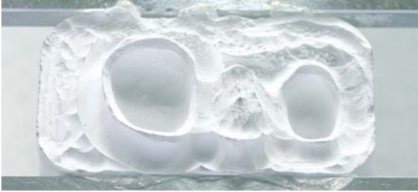
Further detailed internal milling with 2L bur
