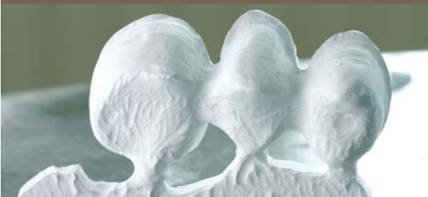
Disconnected bridge with remaining support base – ready for immersion into Colour Liquid
